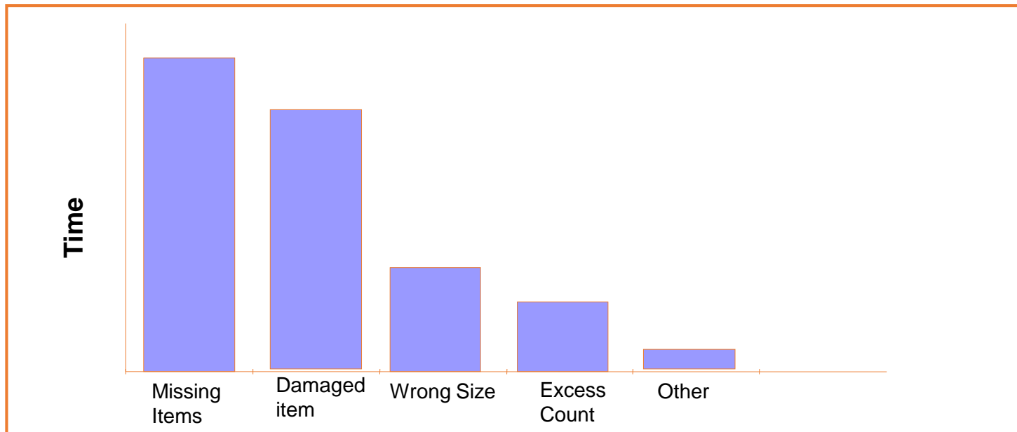
Pareto of Surgical Setup Errors by Time Lost Due to the Error
